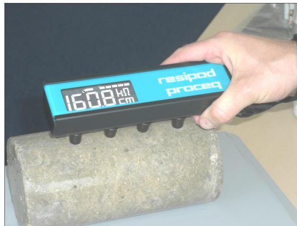
Figure 4 Wenner Array Placement
