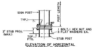
ELEVATION OF HORIZONTAL CONNECTION W SECTION
