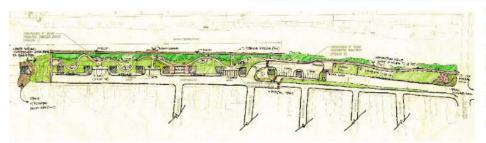
8-foot-wide concrete sidewalk that stretches from the bridge at Grand Caillou Road to the western end of the sidewalk along East Main St. Its design will allow future development of a dog park, kayak launch, parking lots, permanent outdoor exercise equipment, and natural amphitheater. Providence personnel coordinated the project design and grant application and administration, as well as provided topographic surveying and CE&I services with project representation.
