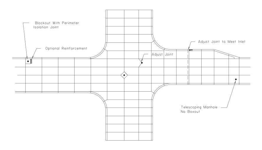
Figure 6-08: Adjusting Joints for Utility Fixtures
