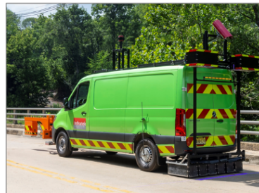
High-Speed Chain Drag, Crack Mapping and Non-Destructive Evaluation High-Speed Visual Inspection No Lane Closure
