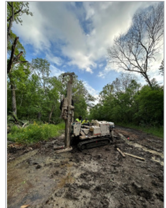
Soil sampling by direct push drilling methods
