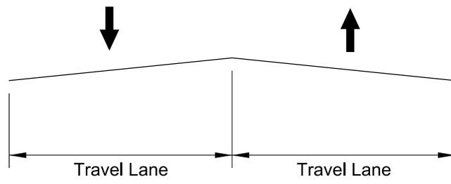
Figure 5-06: Two-Way Tangent Crown
