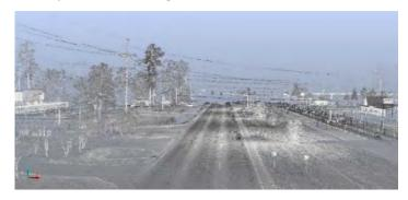
elements were performed in accordance with the latest LADOTD Location and Survey Manual and conformed to the latest standard practices/procedures. All deliverables were in LADOTD required formats. 3D Terrestrial Scanning was used in conjunction with traditional means and methods to complete this project.
