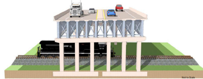
Typical Bridge Section, Norfolk Southern Railroad Overpass.
