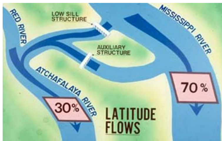
Figure 4. Old River Control Structure Schematic 15
