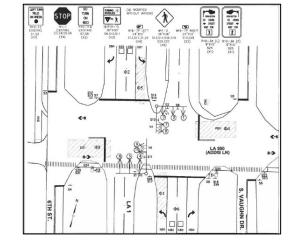
Traffic Signal Construction Plans were performed for LA 1 at LA 990 based on the latest DOTD Traffic Signal Inventory v3.2, DOTD Signal Design Manual, MUTCD & EDSM VI.3.1.6 Section 5. This task included signal timing parameter calculations, signal equipment layout, wiring diagram, DOTD pay items, estimated quantities and construction cost.
