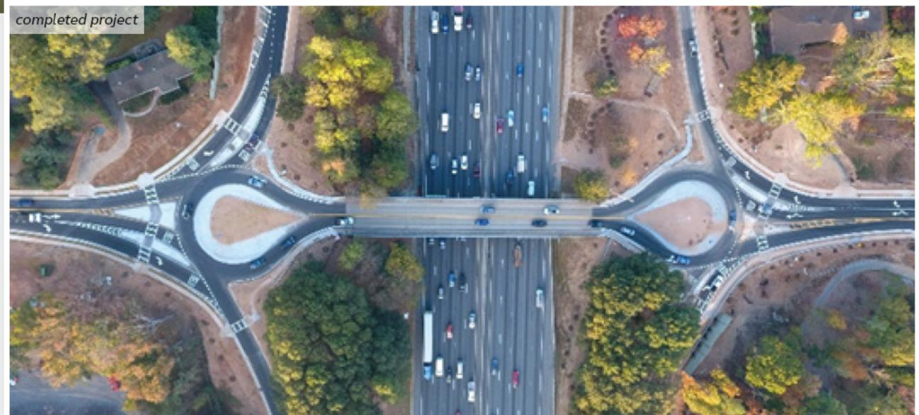
*The Arcadis team has the precise experience in designing skewed and/or non-traditionally shaped roundabout intersections. At off-set intersections, roundabouts can be used to better align approach legs left of center to the roundabout, which leads to improved fastest-path speed control and lane alignments, improving roundabout safety and operations.*
