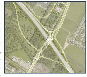
interchange is currently in construction and as previously stated will be the state's first operational Diverging Diamond Interchange (DDI), an innovative approach in interchange design. The Pecue Lane DDI provides a higher level of operational efficiency and is a safer alternative to a conventional diamond interchange. It will consist of three thru lanes in each direction with raised medians and sub-surface drainage.
